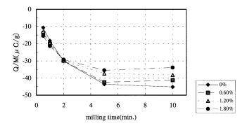
Figure 5.The charge-up behavior of the toners with the various amounts of CCA.
