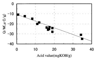
Figure 3. Dependence of Q/M of the toners on Acid Value of polyester.
